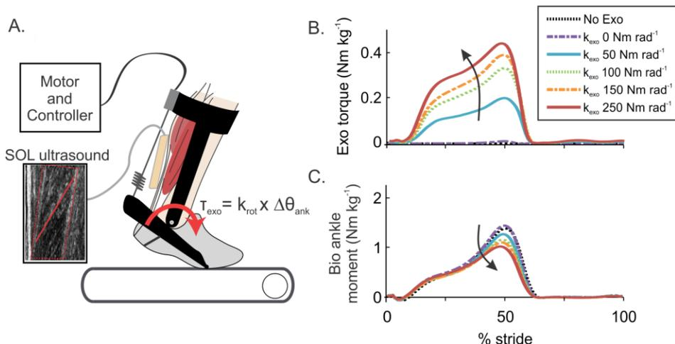
**Figure 1:** (A) Experimental setup. During exoskeleton assisted walking at five stiffnesses, we imaged soleus (SOL) fascicles using B-mode ultrasound. (B) Exoskeleton torque increased with spring stiffness ( $k_{exo}$ ). (C) Biological contributions to the ankle moment, averaged across the 11 subjects and normalized to body mass, decreased with increased exoskeleton stiffness.
