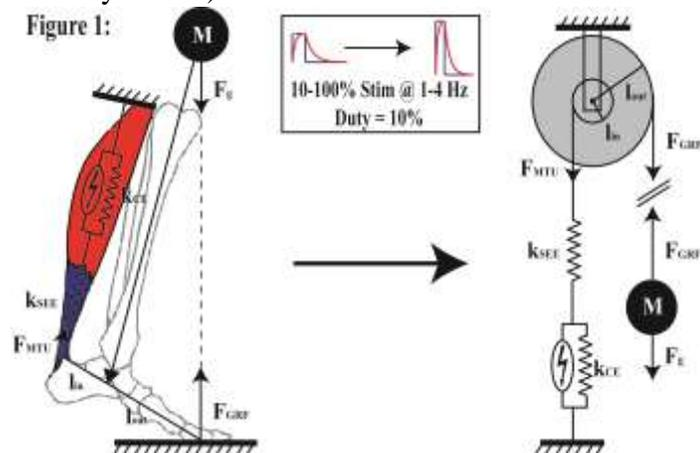
**Figure 1. Lumped ankle plantarflexor MTU model of vertical hopping.** A bodymass in gravity with fixed mechanical advantage ( $L_{in}/L_{out}$ ) simulates ankle MTU dynamics during cyclic contractions. Simulations were performed with series elastic stiffness,  $k_{SEE}$  at baseline ( $180\text{kN/m}$ ),  $k_{SEE}/3$  ( $54\text{kN/m}$ ) and  $k_{SEE} \cdot 3$  ( $540\text{kN/m}$ ).
