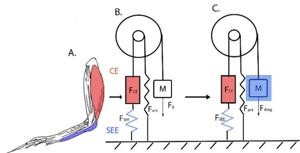
**Figure 1. Bullfrog plantaris (A) is basis for MTU model. (B) Terrestrial environment (C) Fluid environment.** A body mass in gravity operating with a fixed mechanical advantage simulates bullfrog MTU dynamics during cyclic contractions. In terrestrial implementation, gravitational forces dominate (B) while in fluid implementation, drag forces dominate during MTU shortening, and antagonist spring forces return the MTU to longer lengths (C). Simulations were performed with a K value of 1.875.
