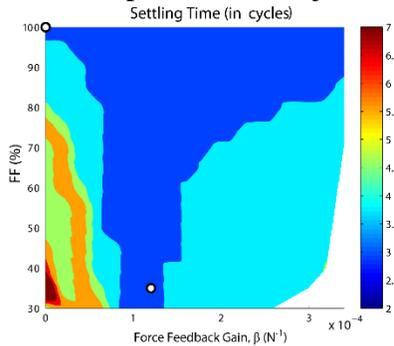
**Figure 1:** Settling time contours as a function of feedforward (FF) contribution and positive force feedback (PFB) gain,  $\beta$ .
