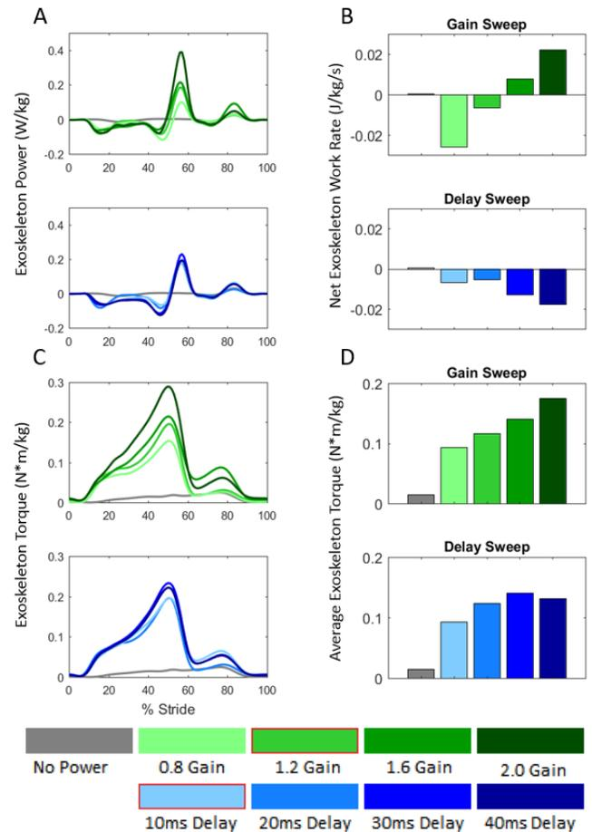
**Figure 2:** In the gain sweep, exoskeleton power (A) and net work rate (B) increased across conditions by increasing the torque profile (C) and average torque (D). In the delay sweep, average torque peaked, before decreasing and net work rate was entirely negative. Darker colors indicate higher values. Red outline indicates base parameters (Gain: 1.2, Delay: 10ms). Curves are study average trajectories.
