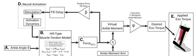
**Figure 1:** Neuromuscular model controller block diagram. Biological force, as computed by the internal muscle-tendon state, is scaled and applied across a moment arm to calculate desired exoskeleton torque.
