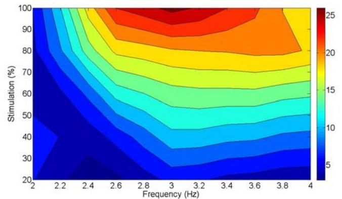
**Figure 3.** Contours of peak *active* contribution to contractile element force (Newtons) as a function of both magnitude and frequency of muscle stimulation. Note that peak active muscle force occurs when stimulated well above the natural frequency of the passive system ( $\sim 2.5$  Hz).
