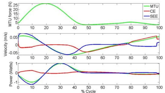
**Figure 1.** Force, velocity, and power generated during a single cycle with a stimulation of 100% and a period of 3Hz. Stimulation is from 0-10% of the cycle. Note significant elastic energy storage and return in the SEE.
