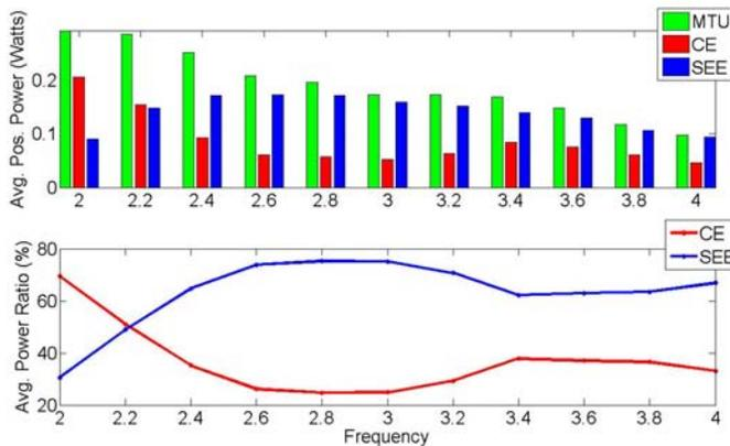
**Figure 2.** Graphs of (top, bars) average positive power output of the muscle-tendon unit (MTU), contractile element (CE), and series elastic element (SEE) and (bottom, lines) Power Ratios -  $CE/(CE+SEE)$  and  $SEE/(CE+SEE)$  versus stimulation frequency calculated over a single contractile cycle.
