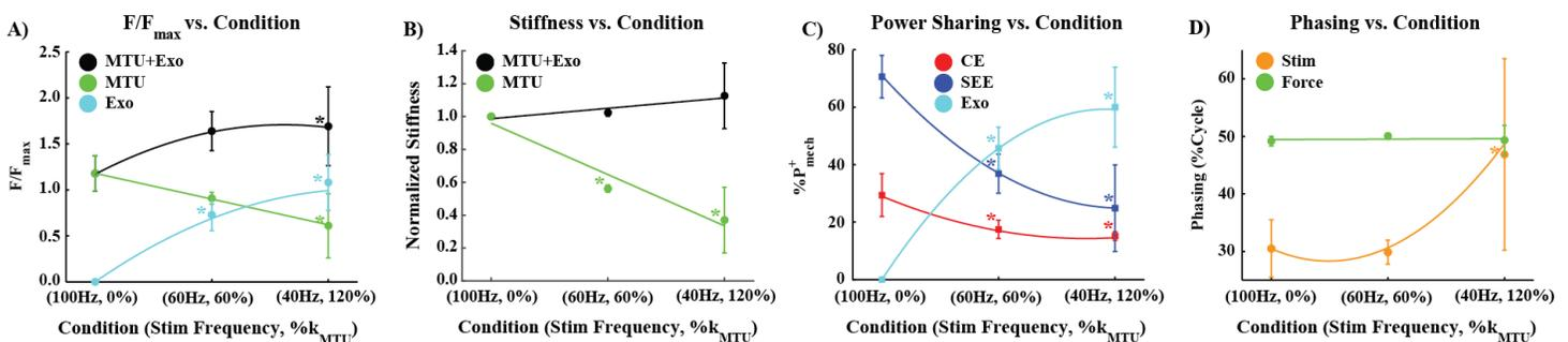
**Figure 2** Plots of **A)** Normalized peak force, **B)** Stiffness, **C)** Sharing of average positive power, and **D)** Stimulation and peak force phasing relative to minimum MTU length. A \* indicates statistically significant variation relative to the unassisted condition.
