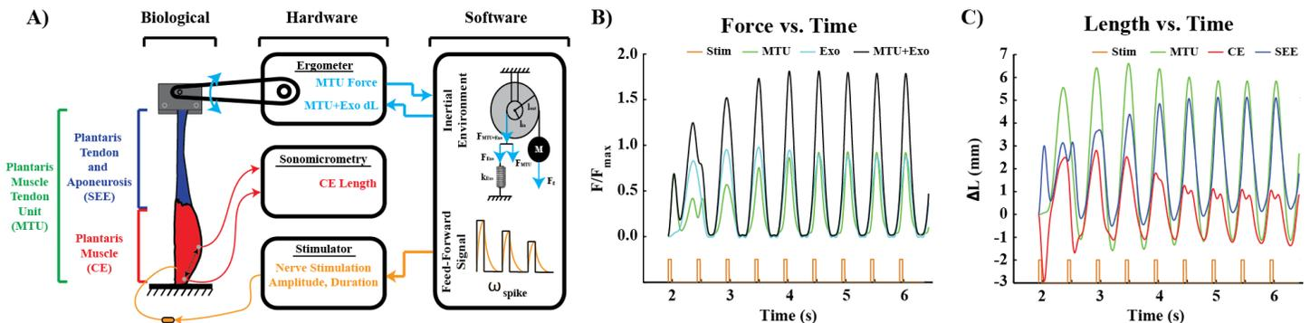
**Figure 1** A) Schematic of experimental setup and control workflow. B) Force vs. time and C) length versus time for a representative trial in the 60Hz, 60% $k_{MTU}$  condition.
