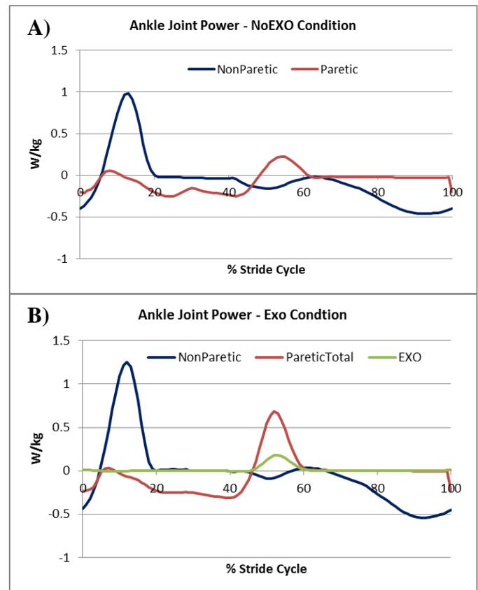
**Figure 2:** The total ankle joint power profiles during the NoEXO condition (A) and the last repetition of the EXO condition (B). The data were averaged from 10 consecutive steps obtained during the last minute of each condition. In the EXO condition, the total paretic ankle joint power (red) contains contributions from both the exoskeleton (green) and the biological muscles (not shown).
