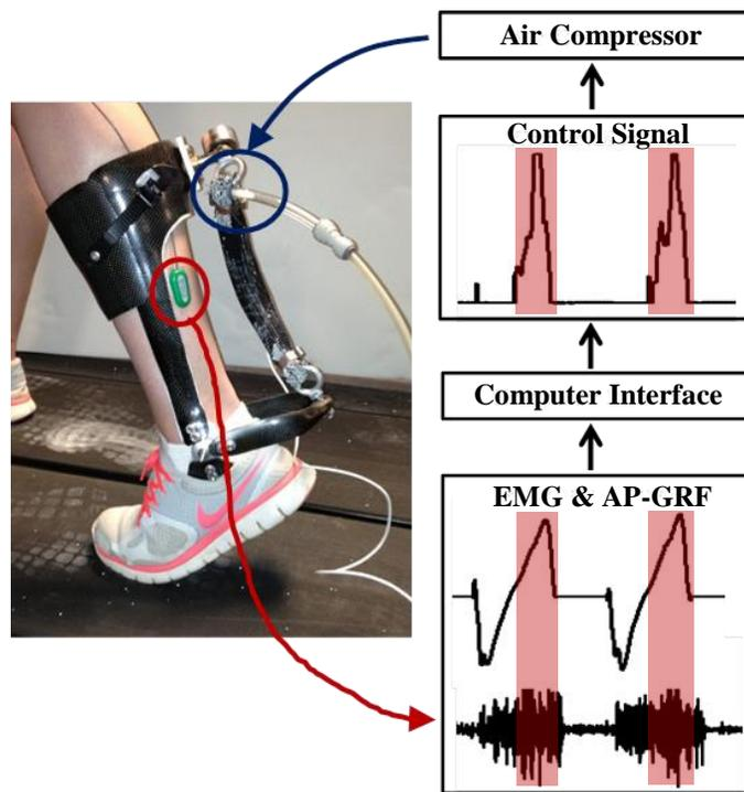
**Figure 1:** The soleus EMG and AP-GRF (from an instrumented treadmill) were collected in real-time to control the magnitude and timing of exoskeleton actuation. The *proportional myoelectric propulsion* (PMP) controller requires soleus EMG amplitude above a set threshold during the propulsive phase of stance, encouraging the user to activate the muscle to receive mechanical assistance.
