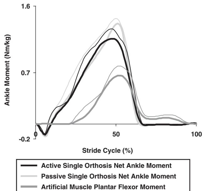
Fig. 7. Net ankle and artificial muscle moments. Mean + standard deviation of net ankle moments and artificial pneumatic muscle moments for the three subjects during over ground walking at 1.0 m/s. Net ankle moments are during the single passive and single active conditions. Artificial pneumatic muscle moments are from the single active condition. Plantar flexion moments are in the positive direction.
